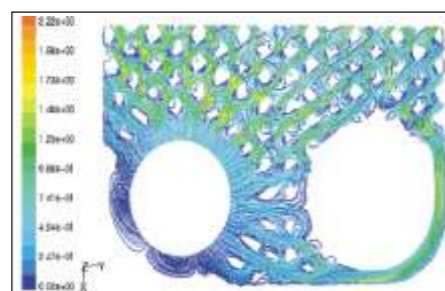
Simulation is one of the most important stages in the development of new and existing CBEs. The ability to evaluate different plate patterns by simulating flow rate and directions offers great opportunities for improved functionality.
